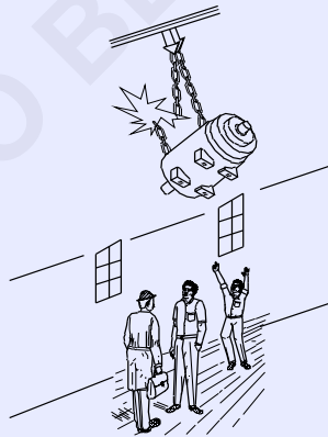
7 STANDING BELOW A SUSPENDED LOAD
